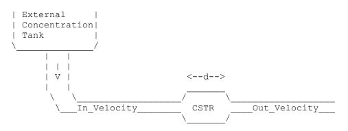
Naturally, the External Concentration field does not contain the actual concentration of the external tank but the concentration the species will become once it is diluted in the CSTR before any reactions occur. A rough approximation of the residence time in a CSTR can be calculated as follows:2 x d (the distance across the CSTR parallel to the in/out flow) / (In\_Velocity+Out\_Velocity). You can have different residence times for different species.
