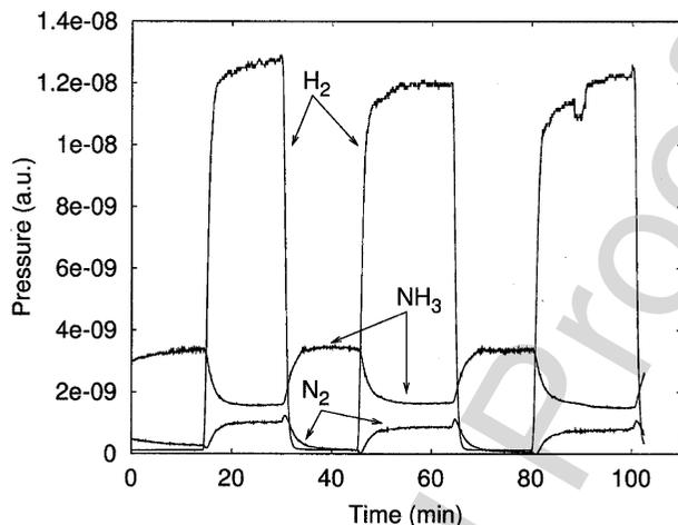
**Fig. 4.** Mass spectrometer results of ammonia decomposition in a microhollow cathode. Ammonia flow is at 1.5 sccm, with an upstream pressure of 100 Torr. The voltage of the plasma is 480 V and the current is 9 mA.
