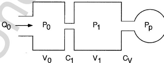
Fig. 11. Two-volume geometry used in lumped conductance model.
