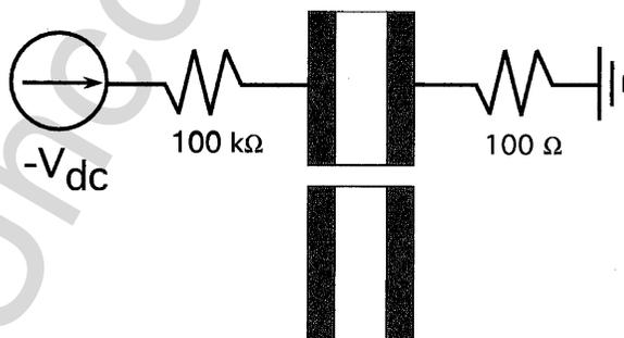
Fig. 1. Microhollow cathode and electrical circuit.
