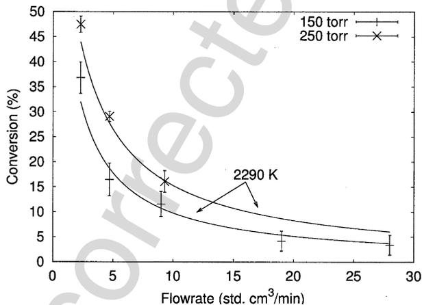
**Fig. 9.** CO<sub>2</sub> conversion as a function of flowrate for two operating pressures. Both sets of data are fit to the same effective reaction temperature.
