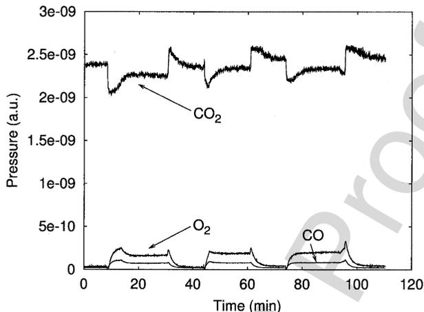
**Fig. 8.** Mass spectrometer signals of carbon dioxide decomposition for 19 sccm, 150 Torr upstream pressure and 5.2 W. When the plasma is on, carbon dioxide decreases, while carbon monoxide and oxygen increase.
