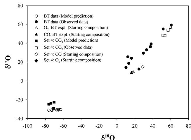
FIG. 6. A three isotope plot showing the oxygen isotopic composition of the product  $CO_2$  in case of set 4 and BT experiments. The average enrichment observed in BT experiments is  $\delta^{18}O=98.1$  and  $\delta^{17}O=64.4$  whereas in set 4 (present experiment) the values are  $\delta^{18}O=128.1$  and  $\delta^{17}O=76.9$ . Lower enrichment observed in BT case could be due to a larger amount of the product  $CO_2$  as compared to that of set 4.
