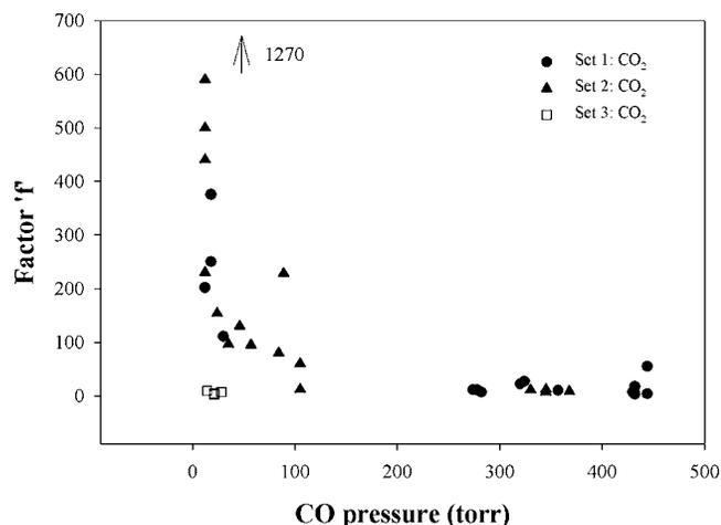
FIG. 5. Variation of factor  $f$  (which enhances  $\text{CO}_2$  production by increasing  $[M]$ ) with pressure.  $f$  increases with decrease in CO pressure suggesting increased importance of surface induced stabilization of  $\text{CO}_2^*$ . For high CO pressure or experiments done in 5 l chamber,  $f$  ranges from 1 to 55 whereas for low CO amount, value of  $f$  could be as high as  $\sim 1270$ .
