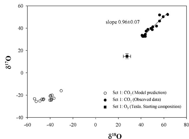
FIG. 1. Oxygen isotopic compositions (in ‰ relative to VSMOW) of product CO<sub>2</sub> (set 1 samples) defining a line with slope of  $0.96\pm 0.07$ . The average  $\delta^{18}\text{O}$  and  $\delta^{17}\text{O}$  values of CO<sub>2</sub> samples calculated from the KINTECUS model are -43‰ and -20‰. Note that CO<sub>2</sub> is enriched in heavy oxygen isotopes in an anomalous fashion.
