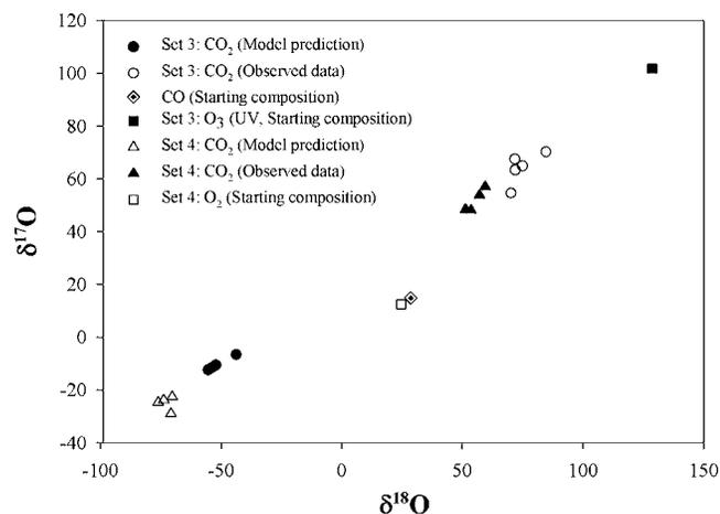
FIG. 3. A three-isotope plot of the experimental data observed in sets 3 and 4 along with results of model simulation. In set 3,  $O_3$ -CO mixture was photolyzed using visible lamp whereas in set 4,  $O_2$ -CO mixture was photolyzed in UV light. The average  $\delta^{18}O$  and  $\delta^{17}O$  enrichments (difference between observed data and model prediction) are (126.8, 74.8) in set 3 and (128.1, 76.9) in set 4.
